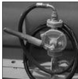
WASTE OIL/SUMP PUMP
